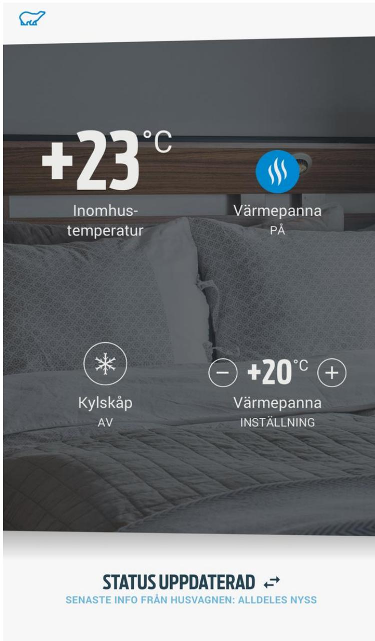
Open Polar connect and make sure that "Värmepanna" is "PÅ" and then set the desired temperature down below. OBS! It's not possible to change the temperature over the value you put in the aldepanel. For example, if the Alde display is set on 24 degrees, you cannot go over 24 degrees in the application.
